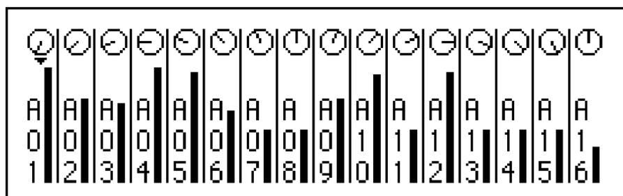
This is a graphic simulation of a multi-channel stereo mixer, showing a simulated volume slider and pan knob for each of the 16 pads in pad bank A (A01-A16).
