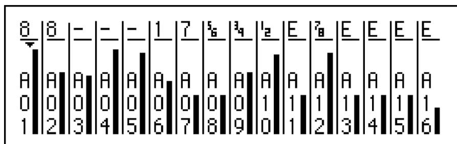
Similar to the Stereo Mix screen, this screen presents a graphic simulation of a multi-channel mixer, showing a simulated volume slider and an output assignment for each of the 16 pads in pad bank A (A01-A16). To view other pad banks, press the PAD BANK key.
