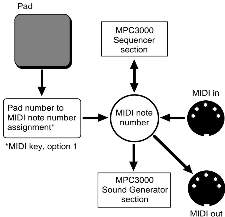
As you can see from the diagram, hitting a pad will generate a pad number, which is then converted into a MIDI note number. This note number can then trigger a sound in the Sound Generator section, be recorded by the Sequencer section, and/or go out the MIDI output. Similarly, note numbers coming in from the MIDI input can trigger a sound and/or be recorded into the sequencer. And note numbers played back by the sequencer can trigger internal sounds and/or go out the MIDI output.
