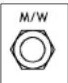
This socket provides a control voltage output relative to the Mod Wheel (Midi CC no1) generated by the Midi master keyboard/controller. There is an internally routed patch (see Midi routing switch note 2).
