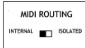
The Midi Routing switch controls the internal routing from the Midi-CV Converter to five control inputs within SPAWN. With the switch in the 'Internal Routing' position the following internal patches are made.
