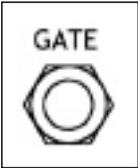
This socket provides the output for the Midi generated gate. When no key is pressed on the controlling keyboard no voltage appears at this socket, when a key is pressed (anywhere) on the keyboard approx 10 volts will be available at this socket. It remains at this level while the key is held and drops back to OV on release of the key. This 'gate' initialises the envelope generator.
