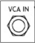
This is an external input that allows audio and control signals to be processed by the VCA.
