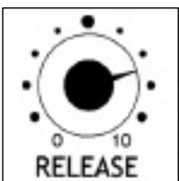
The Release knob controls the amount of time it takes the output voltage to fall to '0' once the gate has ended.
