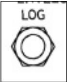
This input allows logarithmic modulation of the VCA by an external source.
