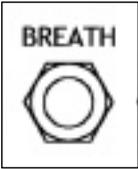
This socket provides a control voltage output relative to the breath controller (Midi CC no2) generated by a Midi controller. This is a bi-polar controller e.g it can produce +ve and -ve voltages in the range of +/- 5volts.
