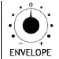
The Envelope knob alters the cut-off point according to the set up of the envelope generator allowing automated shaping of the filter negatively and positively.
